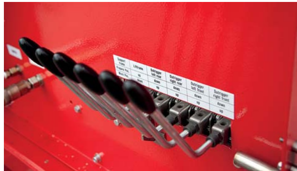
Control panel on base frame
