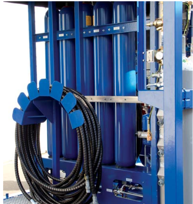
Hydraulic storages and hoses
